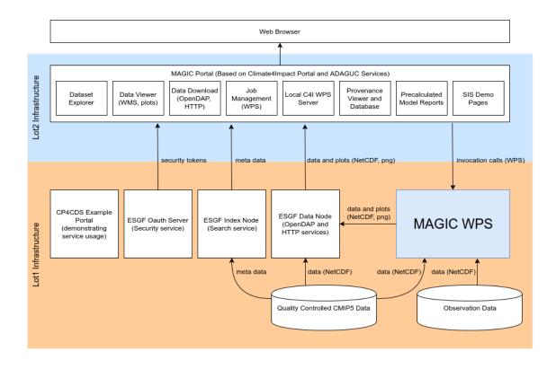
This is an overview of the infrastructure in which the WPS is running. It consists of the portal system based on Climate4Impact and ADAGUC Services. These run on cloud infrastructure outside of ESGS, and is managed by the MAGIC team.
